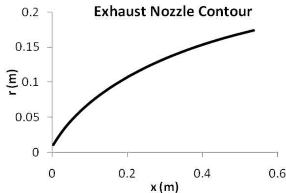
**Fig 5 Exhaust nozzle contour design based on Rao's methods.**
