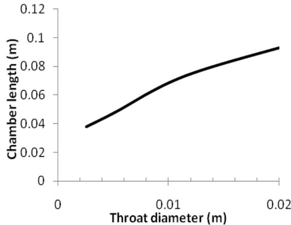
**Fig. 4 Relation between chamber length and throat diameter; adopted from [Huzel and Huang, 2004].**
