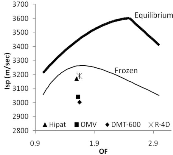
**Fig. 2 Variation of vacuum specific impulse with OF ratios; Hipat, OMV, DMT-600, and R-4D are the  $N_2O_4/MMH$  upper-stage / spacecraft engines in operation.**
