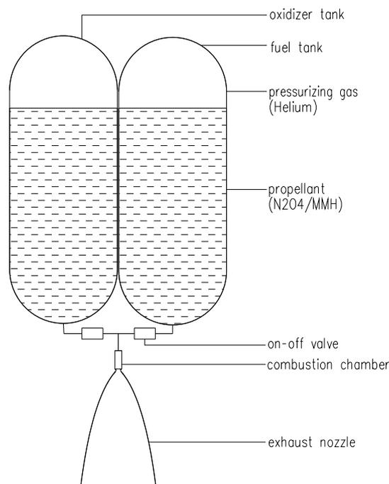
**Fig. 1 Gas pressurized N<sub>2</sub>O<sub>4</sub>/MMH liquid propellant rocket engine.**
