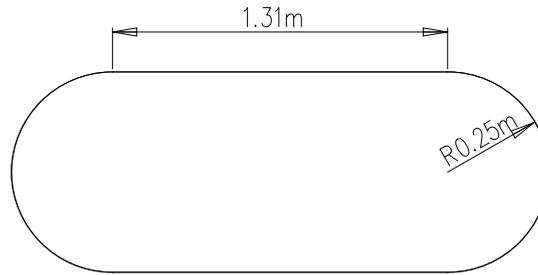
**Fig. 3 Fuel tank and oxidizer tank internal dimensions.**
